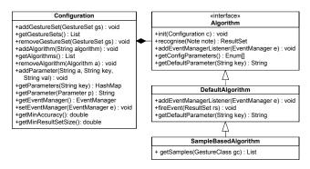
Figure 2. Algorithm class diagram
