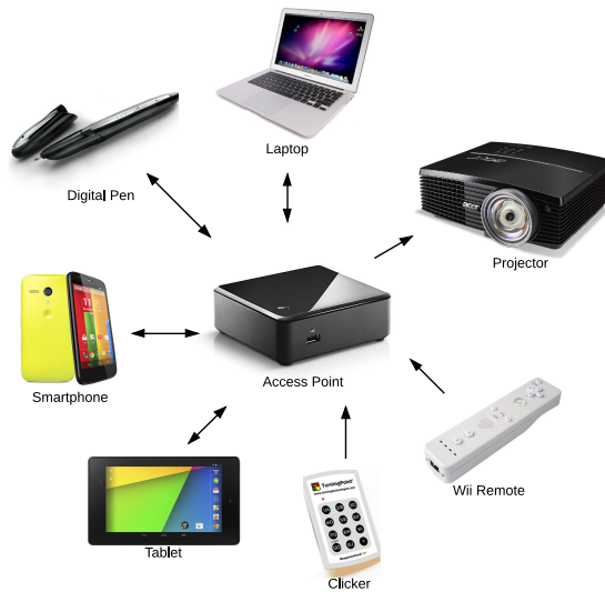
Figure 6.3: The MindXpres access point orchestrates and mediates communication between presentations, plug-ins and hardware peripherals
